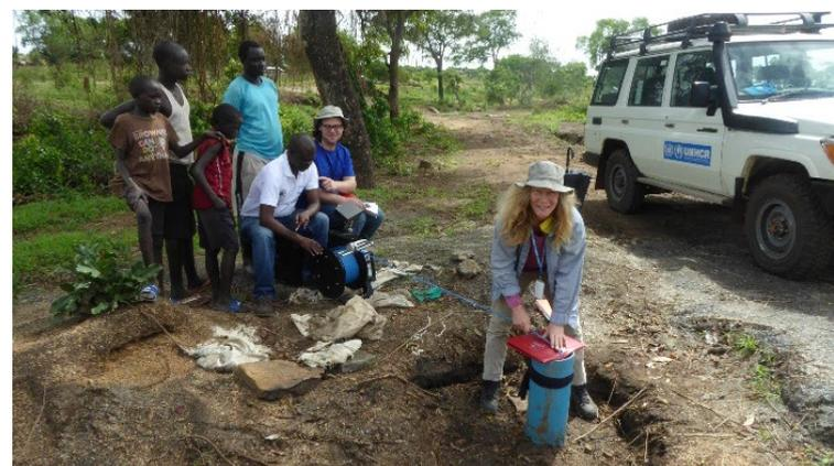
Demonstration of the borehole camera in one of the high-yielding wells which was implemented using the rapid mapping technique
