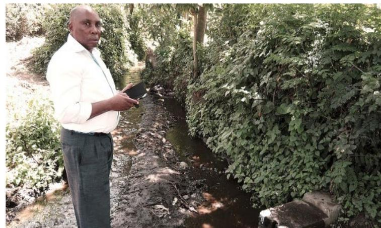
Tito Kitomari taking a discharge measurement with the smart phone app developed by the project (discharge.ch).
